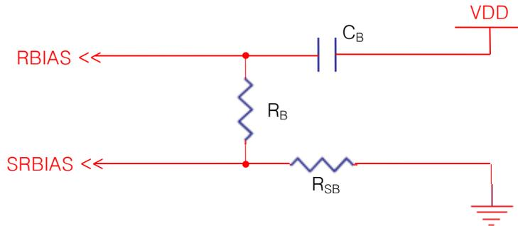
The RBIAS is connecting to the resistor to decide the oscillator and internal bias current. The sensing frequency, internal clock frequency and current consumption are therefore able to be adjusted with  $R_B$ . A voltage ripple on RBIAS can make critical internal error, so  $C_B$  is connected to the VDD (not GND) is recommended. (The typical value of  $C_B$  is 820pF and the maximum Value is 1nF.)
