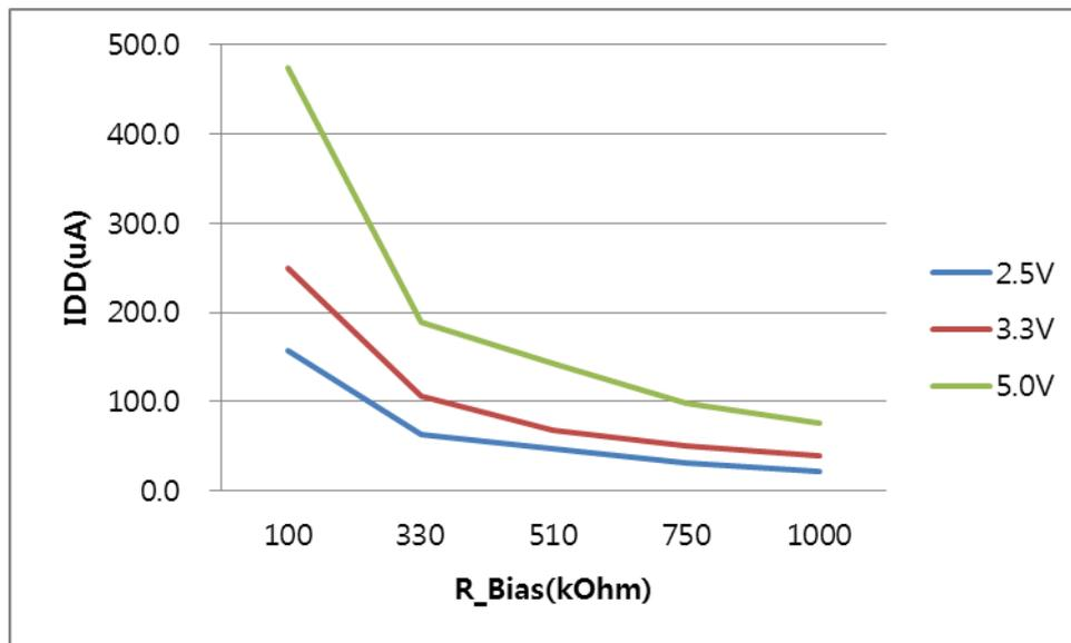
The current consumption curve of TSM12 is represented in accordance with  $R_B$  value as above. The lower  $R_B$  requires more current consumption but it is recommended in noisy application. For example, refrigerator, air conditioner and so on.
