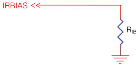
The R<sub>IB</sub> is only charged in making the I2C internal clock and should be implemented as above figure. The smaller R<sub>IB</sub> will increase the I2C internal clock frequency and current consumption (Refer to the following consumption curve).
