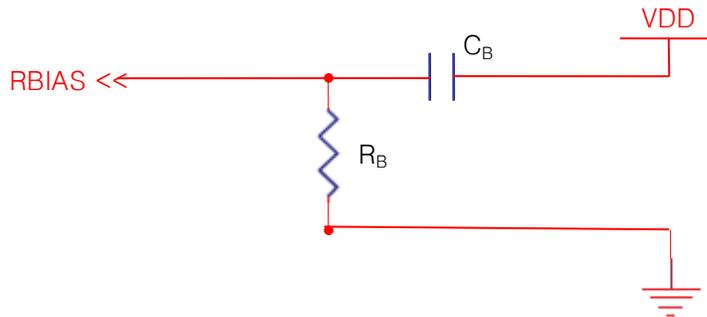
The RBIAS is connecting to the resistor to decide the oscillator and internal bias current. The sensing frequency, internal clock frequency and current consumption are therefore able to be adjusted with  $R_B$ . A voltage ripple on RBIAS can make critical internal error, so  $C_B$  is connected to the VDD (not GND) is recommended. (The typical value of  $C_B$  is 820pF and the maximum Value is 1nF.)
