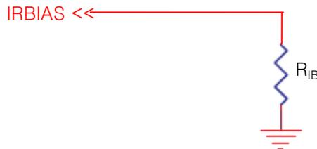
The  $R_{IB}$  is only charged in making the I2C internal clock and should be implemented as above figure. The smaller  $R_{IB}$  will increase the I2C internal clock frequency and current consumption. (Refer to the following consumption curve)
