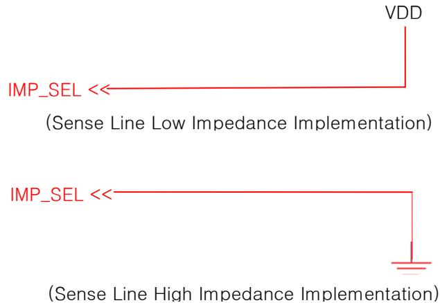
The sense input impedance might be selected by the IMP\_SEL pin. In case of multi channel touch sensor application, the sense lines could be drawing side by side with very small gap. In this case, the sensitivity could be affected by the neighbor channel during out of scanning. Therefore the connection of IM\_SEL pin is recommended to connect with VDD (low impedance mode). In the other case, the high impedance mode (connection with GND) has an advantage for sensitivity.
