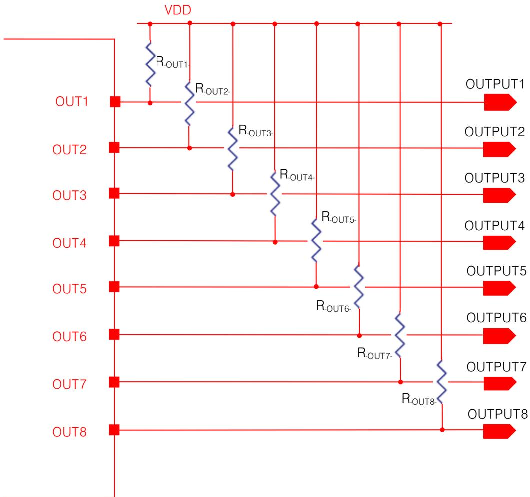
The OUTPUT pins have an open drain structure. For this reason, the connection of pull-up resistor  $R_{OUT}$  is required between OUTPUT and VDD. The maximum output sink current is 4mA, so over a few k $\Omega$  must be used as  $R_{OUT}$ . Normally 10k $\Omega$  is used as  $R_{OUT}$ .
