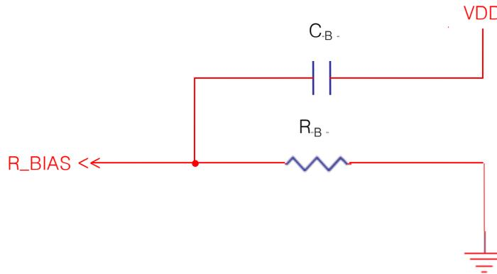
The R\_BIAS is connected to the resistor to decide the oscillator and internal bias current. The sensing frequency, internal clock frequency and current consumption are therefore able to be adjusted with R<sub>B.</sub>. A voltage ripple on R\_BIAS can make critical internal error, so C<sub>B.</sub> is connected to the VDD (not GND) is recommended. (The typical value of C<sub>B.</sub> is 820pF and the maximum Value is 1nF.)
