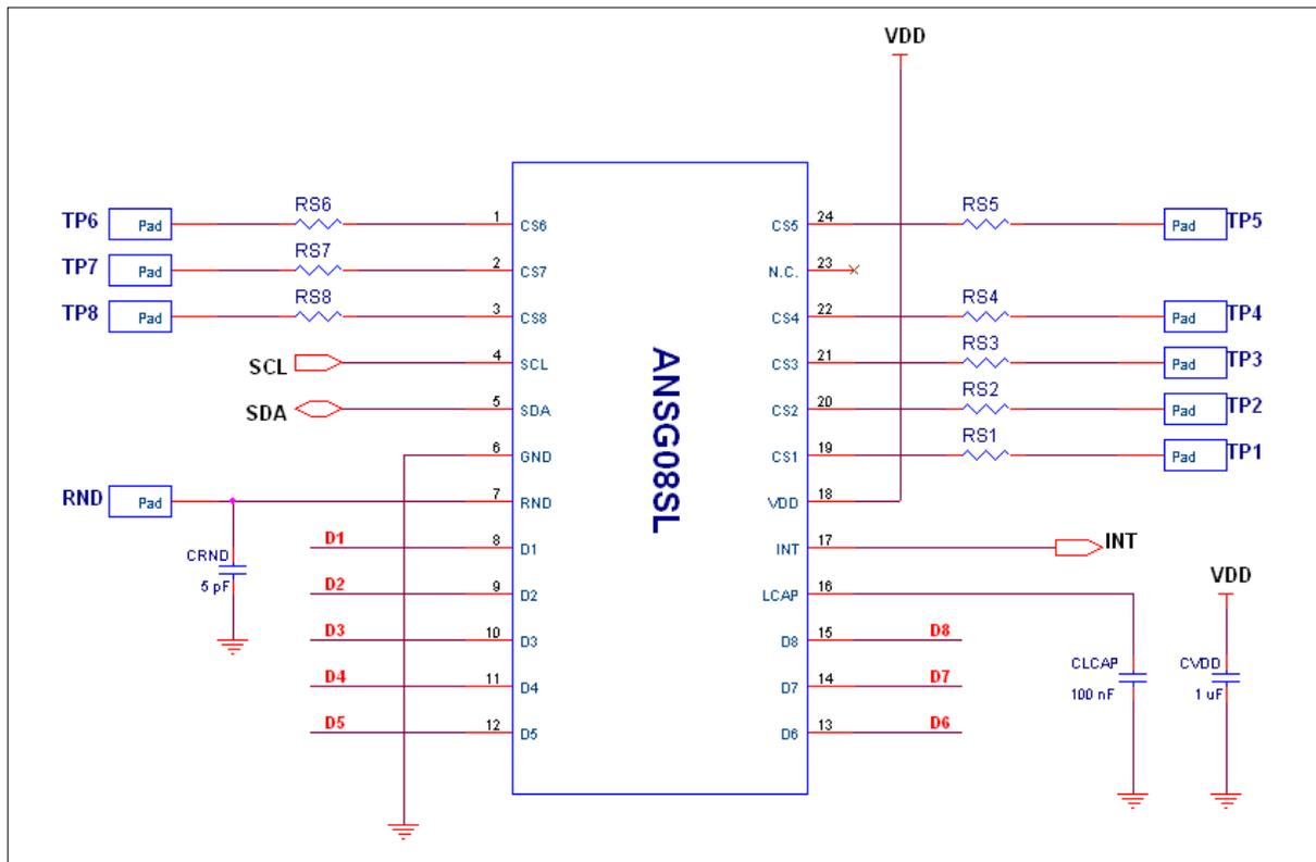
ANSG08SL (24 SOP) Application Example Circuit
