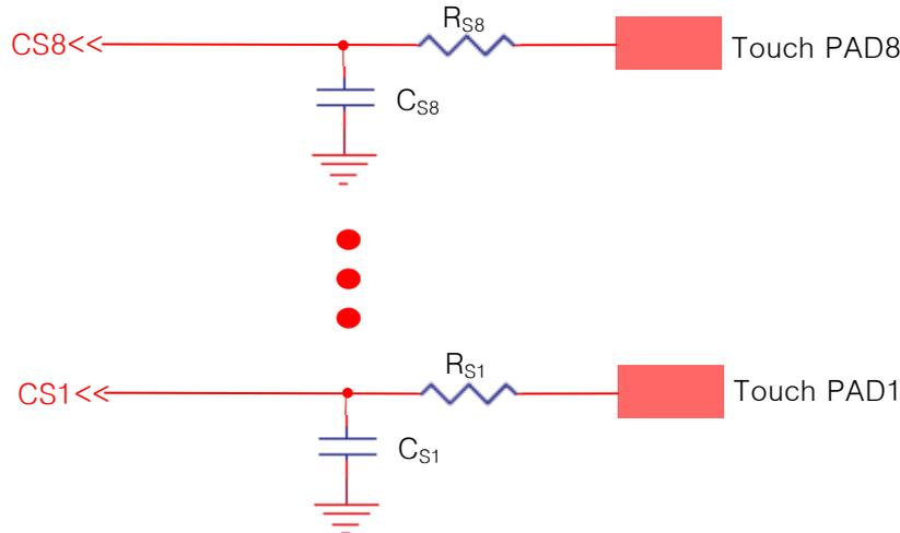
The ANSG08 has eight independent touch sensor input from CS1 to CS8. The internal touch decision process of each channel is separated from others. Therefore eight channel touch key board application can be designed by using only one ANSG08 without coupling problems.
