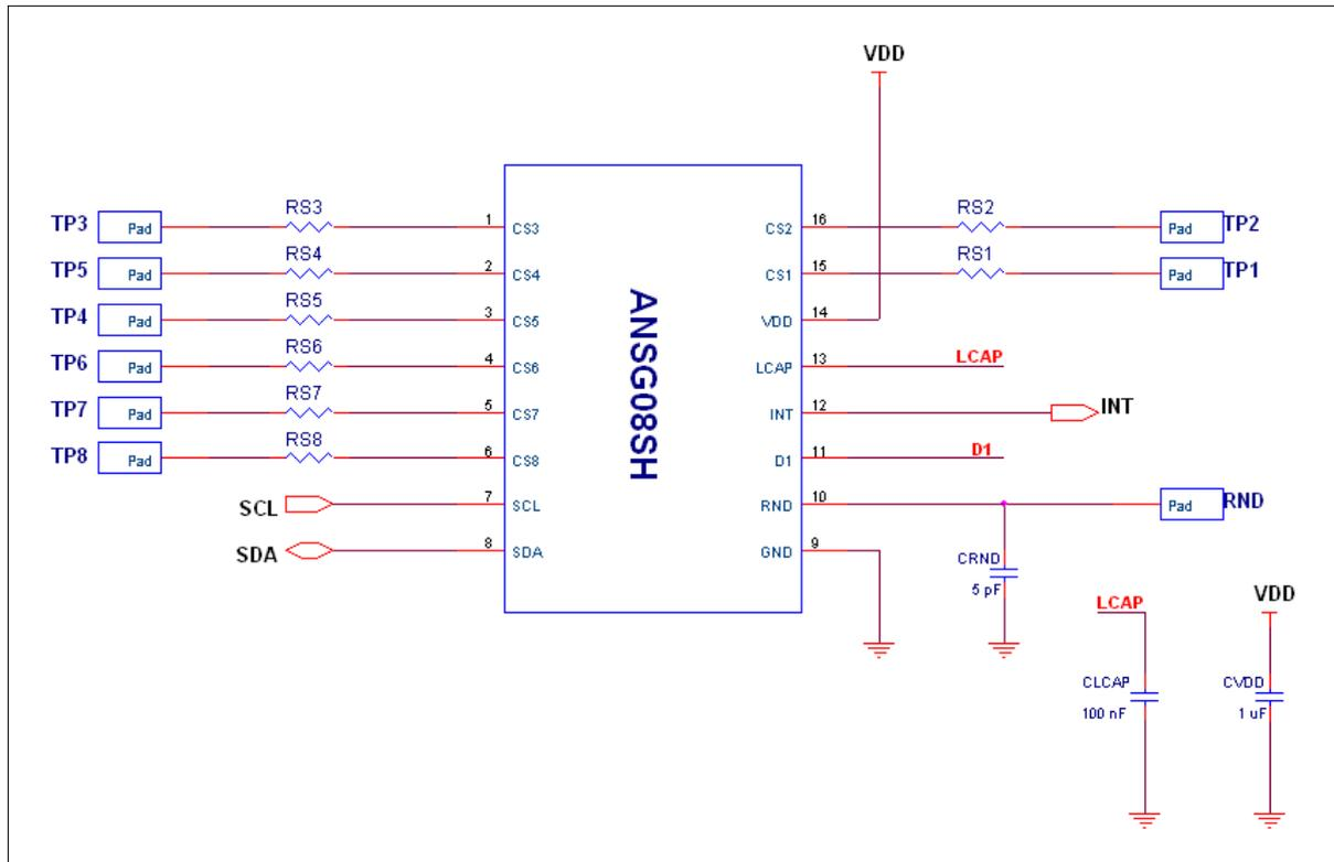
ANSG08SH (16 SOP) Application Example Circuit
